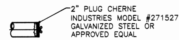
2" PLUG EXISTING LINE TYPICAL
